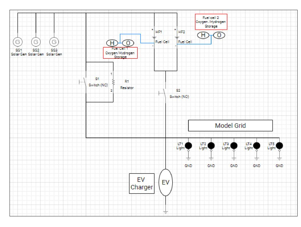
• Our load for this concept was both a heavy drawing load such as the EV charger and physical lights to visually see power transfer.
