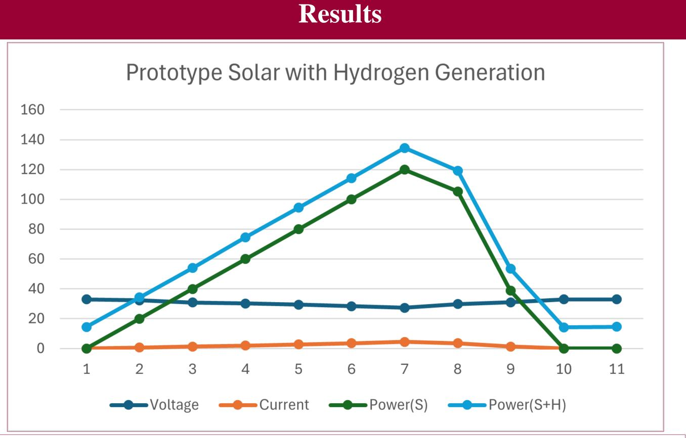
In the graph above, we can see the power output of both the pure solar generation and solar with hydrogen generation. We determined that the hydrogen fuel cells provided a 11.5% - 12.5% increase to the maximum load that the solar cell can handle on its own. With this result, we can safely say that we can effectively eliminate the solar duck curve as long as the peak of the duck curve is no higher than 12% of the solar generation at that given point.
